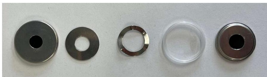
Figure 1. Photo of the un-assembled coin cell with front and back windows, spacer membrane, and the V-loading used for the XANES experiments at DELTA beamline 10.
