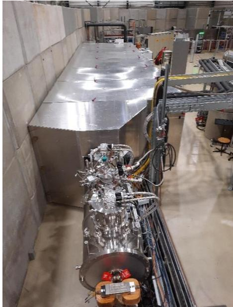
Figure 3: Radiation shielding hutch enclosing the new outlet chamber and the three hard x-ray beamlines.
