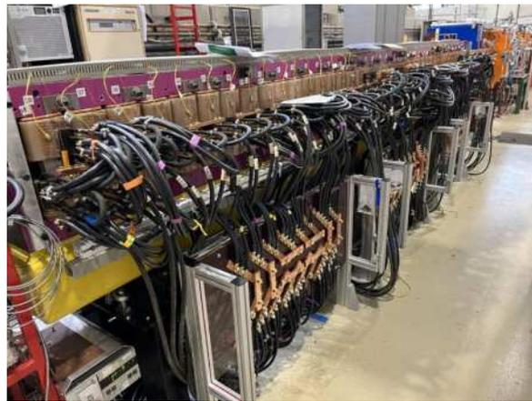
Figure 2: Rewired undulator U250 with three new switchboards in front of it.
