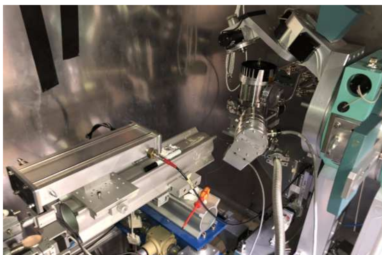
Figure 1: Integration of the DC-sputtering chamber into the Beamline 10.
