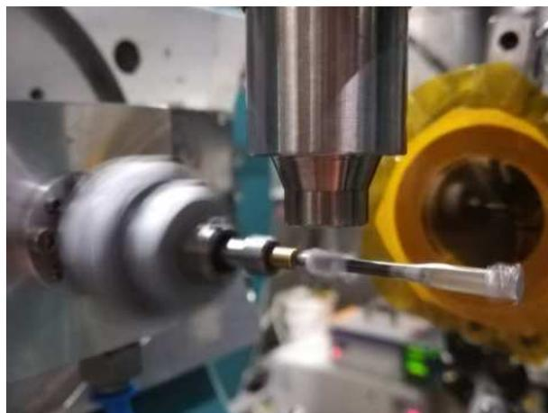
**Fig. 2.** Sample inside borosilicate capillary spun via pressured air during measurement to reduce anisotropy effects.
