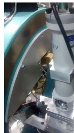
Figure 1: The cryostat is mounted on a Huber Z-stage and connected to the diffractometer via ball bearings to minimize vibrations to the system.
