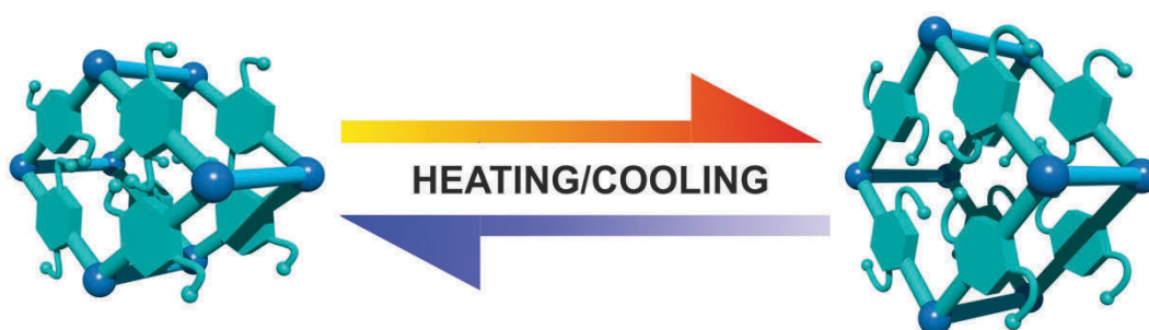
Figure 1: Schematic depiction of the reversible structural transformation of MOFs of the type [M_2(\text{BME-bdc})_2(\text{dabco})]_n as a response to a heating/cooling cycle.
