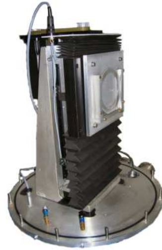
(b) Scanner used to move the wafer and the mask across the beam
