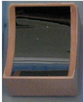
Figure 2: Photo of a doubly-curved crystal in Johann geometry. (Size \approx 25 mm x 30 mm)
