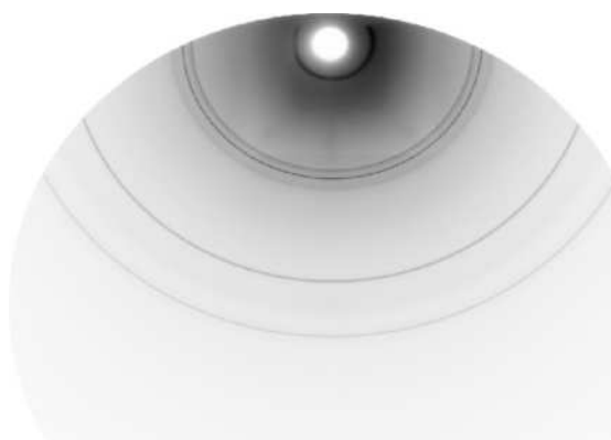
Fig. 1. 2 dimensional picture of x-ray diffraction from CdSe NW
