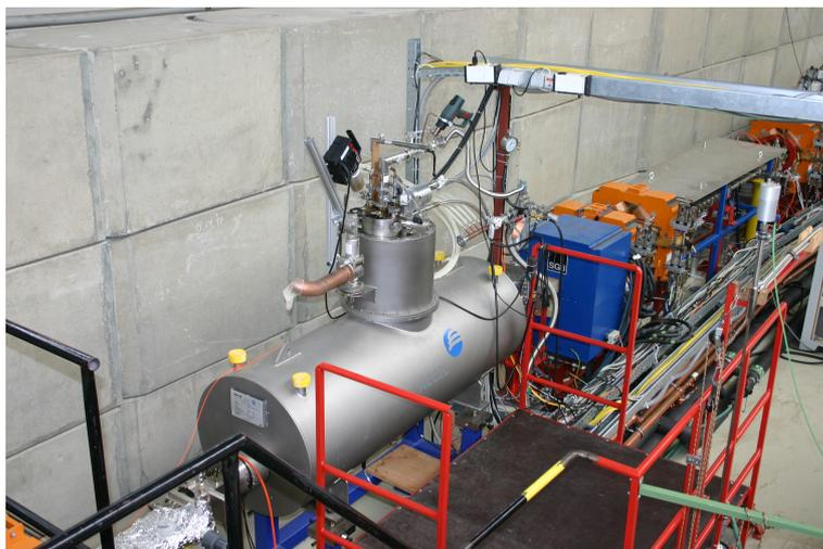
**Fig. 4.1:** *Superconducting Asymmetric Wiggler (SAW).*
