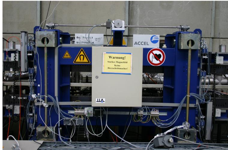
**Fig. 5.8:** Permanent magnets undulator U55.
